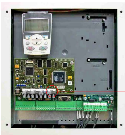
Figure 6-41 COM-8x circuit board (A) in a DCS800 converter (ED7Y type) and a detail of channel CH0 (B) on the board
