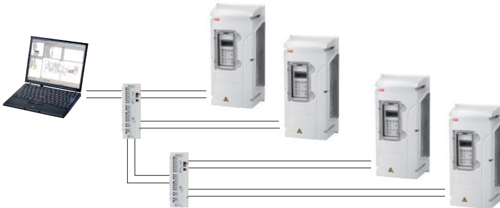
DDCS tree network with optical branching units. PC uses USB or PCMCIA adapter.
