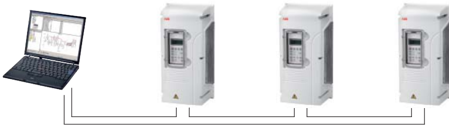
DDCS ring network. PC uses USB or PCMCIA adapter.
