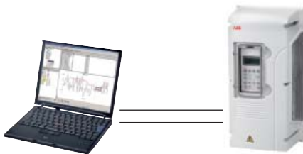
DDCS point to point network. PC uses USB or PCMCIA adapter.
