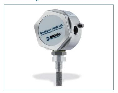
The Easidew PRO I.S. is a rugged instrinsically safe 2-wire dewpoint transmitter for trace moisture measurement in liquids and gases. It is certified for use in IS Class 1 Div 1 Groups A,B,C and D, Ex II 1G EX ia IIC T4 and I.S. I 1 ABCD T4 (Ta = +60°C) hazardous area locations.
