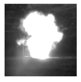
The image to the left shows a hydrogen explosion in near-infrared. The hydrogen fire is easily seen on the video.
