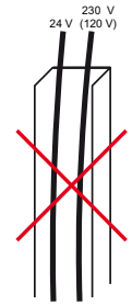
Not allowed unless the 24 V DC cable is insulated for 120/230 V AC or insulated with an insulation sleeving for 120/230 V AC .
