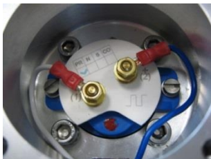
2 wire preamp (Standard / NAMUR)
