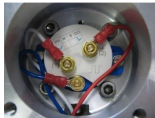
3 wire preamp (Open Collector)
